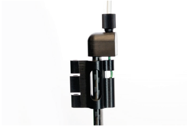
Figure 3-8 Z-Drive at Top Position With Gap
