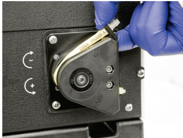
Figure 7-4 Removing the Peristaltic Pump Tubing Cartridge
