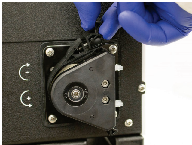
Figure 7-3 Releasing the Peristaltic Pump Shoe
