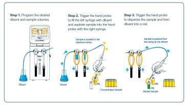
Figure 1: Schematic illustration of the dual syringe dilutor method
