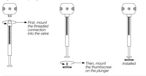
**Note:** The syringe is required to be installed parallel to the face of the PSD/6 or damage will result to the syringe and/or valve.
