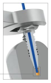
MarvelX UHPLC fittings do not depend on ferrules. They seal at the bottom of the port, without complex techniques, which significantly reduces required torque and enables many more connects and disconnects. Furthermore, they are virtually impossible to over-tighten by hand, limiting wear and increasing product life. An enhanced proprietary tip design also ensures zero dead volume (ZDV) and better chromatography results.
