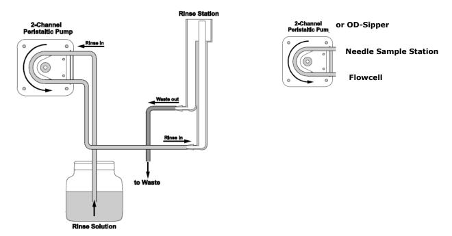
Fitting and adapter kit for sample path - inlet & outlet peristaltic pump (1/16" OD capillary & 1/8" ID tubing)
