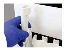
Connect waste tubing to the rinsing station. Engage the rinsing station into the holder. Connect the waste tubing with a waste container. The waste container must be lower than the sampler
