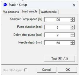
**Pump Speed:** Can only be set if the sample station pump is used as the
