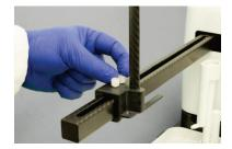
Slide the sample needle unit onto the arm up to the slide and fasten it with the two screws.
