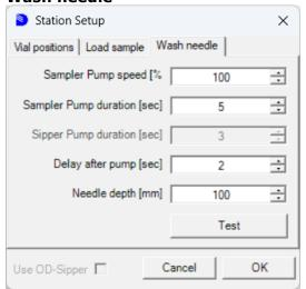
**Sampler pump Speed:** Speed of the sample station pump when washing
