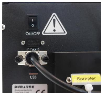
**Attention!!!** The USB-RS232 adapter cables are not ordinary USB-RS232 adapters. The software works exclusively with these cables. The cables are assigned to the devices and must not be interchanged.
