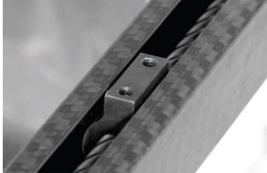
Find the Y-axis carriage on the arm of the autosampler. The Z-drive will be attached to this carriage.
