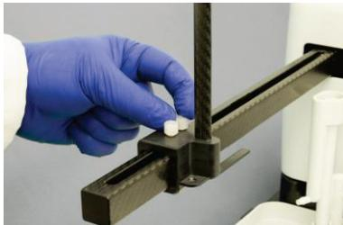
Secure the Z-drive to the carriage using the two thumbscrews.
