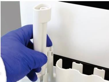
Connect waste tubing to the rinsing station. Engage the rinsing station into the holder. Connect the waste tubing with a waste container. The waste container must be lower than the sampler.
