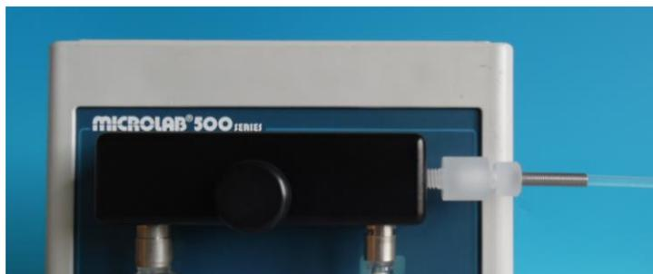
Connect the tubing of the sample needle of the sampler with the right valve of the ML600 respectively the right side of the ML500 Valve. (Pictures of tube connectors are similar and may vary depending on the system) Please note that the tube fittings have ¼-28 threads. In case of a ML500 an adapter (P/N P-694) must be used to convert from M6 thread to ¼-28.
