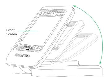
As shown above, the controller can tilt at different angles for user comfort and preference, in addition this controller may also be hung on a wall.
