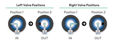
**Note:** The left and right valves can move independently of each other, as indicted in the diagram above.
