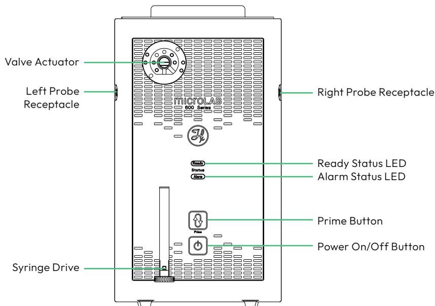
Figure 2-2 Front View of the Dual Syringe Drive Unit
