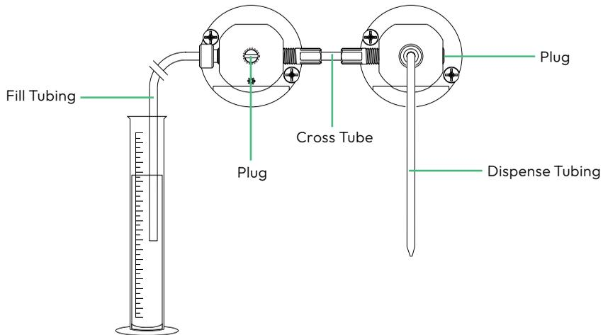
Figure 2-9 Dual Syringe Dispenser Valve and Tubing Assembly
