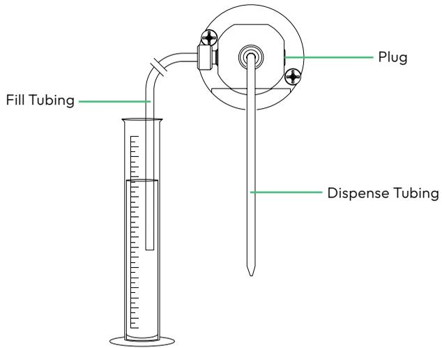
Figure 2-8 Dual Syringe Diluter Valve and Tubing Assembly
